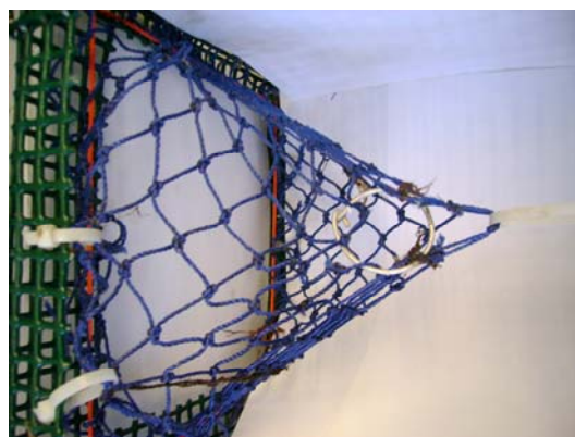
Figure 17. Fike Trap 2 Head Opening. Wire ring creating the size of the entry, 1.5 inches, view from above.
