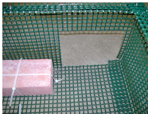
Figure 3. Sample Trap with Head Removed. View from top with lid open. By building the trap and the heads separately, the heads can be changed without major construction.
