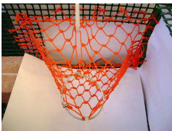
Figure 12. Fike Trap 1 Head Opening. View from above, cloth mesh head with wire ring hoop creating the entry point size, 2 inches. Zip ties hold head in place.
