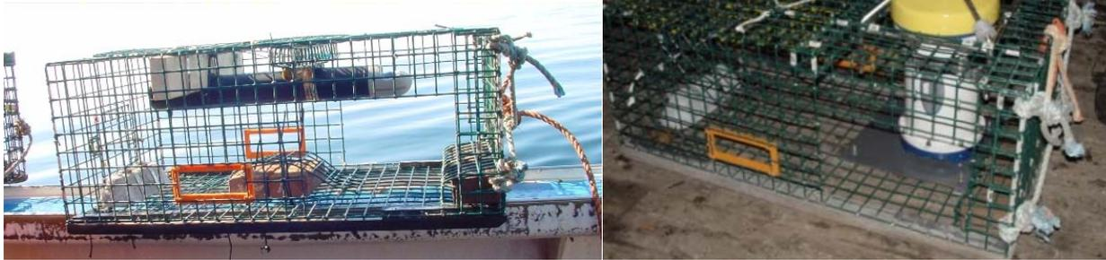
Figure 4 – the Aquadopp acoustic Doppler current profilers from NMFS (l) and GoMOOS (r)
