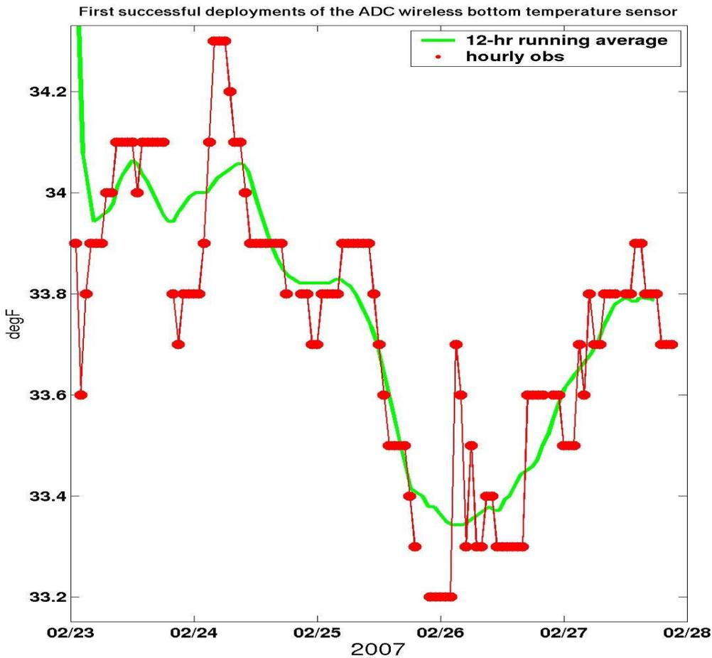
Figure 8. Time series of ADC realtime probe after deployment in Feb 2007 and a wireless download.
