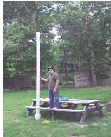
*Figure 5. DATIS surface buoy proposed to house radio beacon.*
