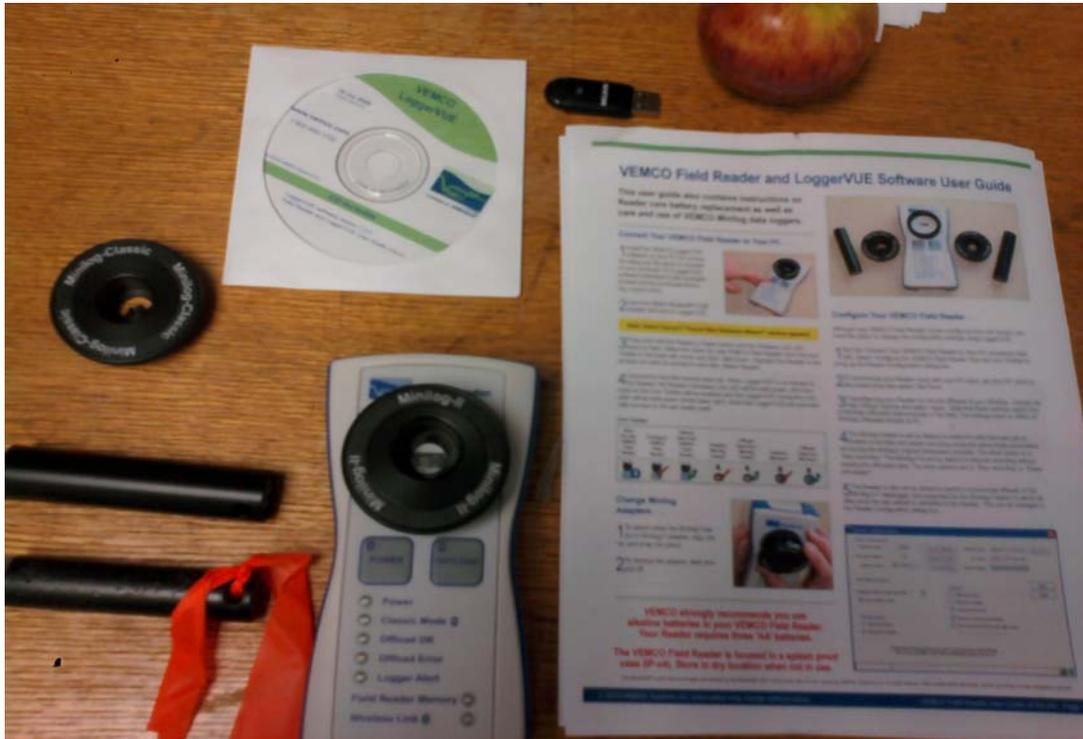
Figure 7. VEMCO's Minilog-II and field reader solution for wireless downloads from the field.
