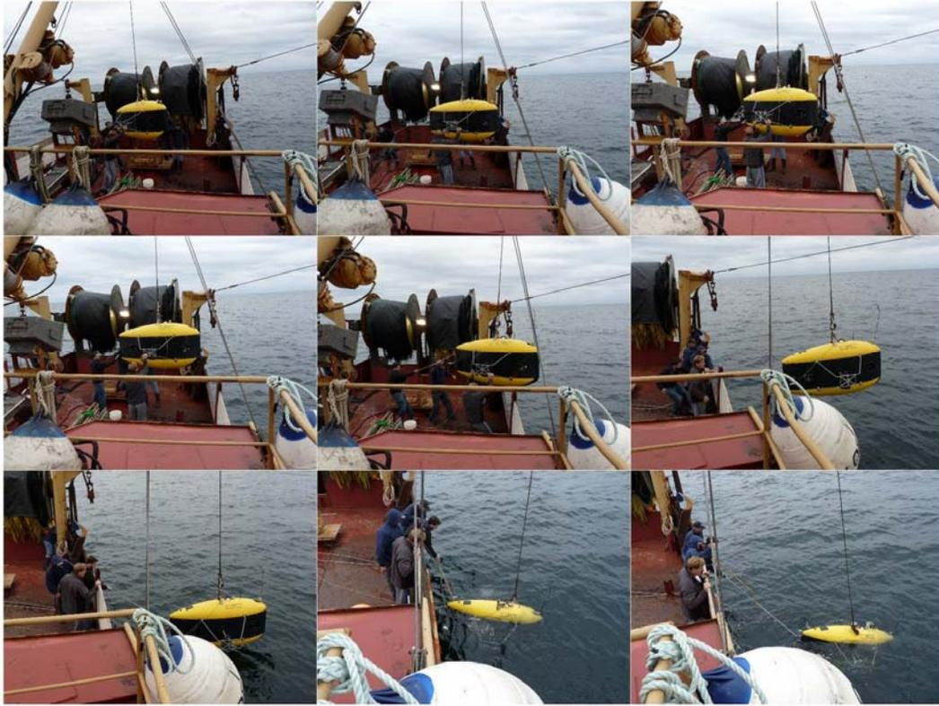
Figure 2: Photographic sequence of a routine deployment of the Odyssey IV from the F/V *Isabella & Ava* using the overhead boom crane. Field operations were conducted at Stellwagen Bank in October 2009.
