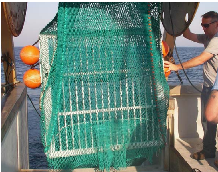
Figure 4: The final white grate mounted in the net's extension.
