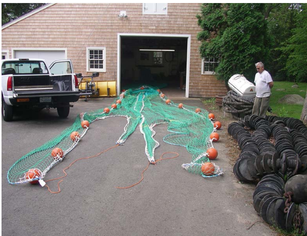
Figure 5: The new raised footrope whiting net used.
