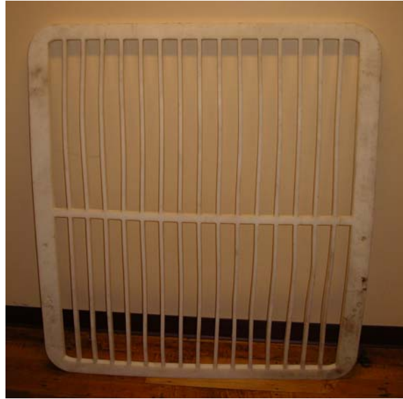
Figure 2: The grate used during the pre-trials. Warping of the bars is evident.
