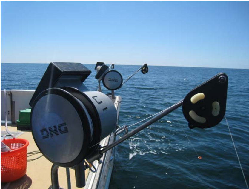
Figure 5. Jigging machines installed on F/V Andanamara. Three machines were deployed off the port rail and stern quarter.
