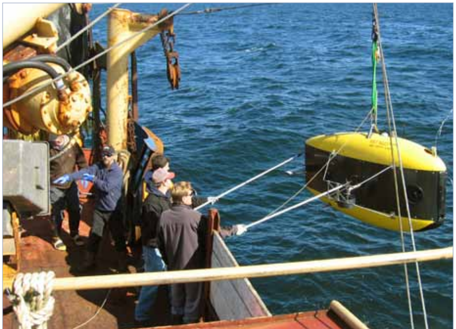
Deploying an Autonomous Underwater Vehicle to study sea squirt. Photo by R. Feeney
